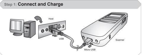
Insert the Micro USB connector into the port on the scanner and the standard USB connector of the USB cable into a USB port on the host PC.
