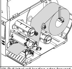
(3) Pull label roll leading edge forward through the media guide bar, damper, media sensor and place the label leading edge onto the platen roller.
