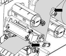
(4)Adjust the label guides to fit the width of the label.
