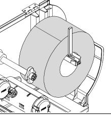
(2) Place the roll of media on the label supply spindle. Flip up the label roll guard. Move the label roll guard horizontally to gently fit the width of label roll.
