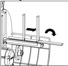
Move the label roll guard horizontally to the end of label spindle then flip down the label roll guard.
