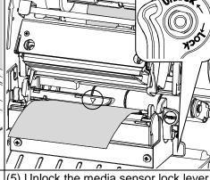
(5) Unlock the media sensor lock lever to adjust the media sensor position and lock the media sensor lock lever. (see note below) (6) Close the print head mechanism by pushing the both sides of print head mechanism. Make sure the latches are engaged securely.
