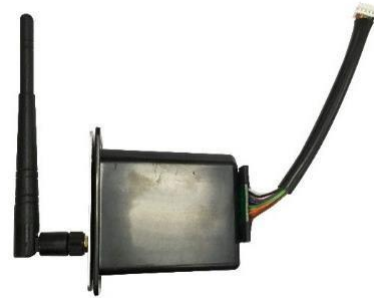
Slot-in Wi-Fi module with antenna and transfer board
